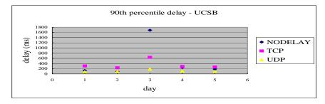
The performance of UCSB varies across measurements. Though most of the time, the performance of UDP is better than that of TCP NODELAY, and the performance of TCP NODELAY is better than that of TCP, there is an exception. On the third day, the delay of TCP NODELAY is abnormally high. It is 1.7 seconds, almost ten times of other days' delay.
