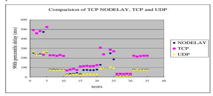
From this chart, we can see that the performance of TCP is the worst. TCP NODELAY and UDP are very close, especially on those stable node pairs. However, on those unstable node pairs, the performance of UDP is much better than that of TCP NODELAY.
