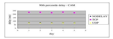
The network from Cambridge to Columbia is very stable. In all five days of experiments, both delay and jitter are very stable without obvious variation. The results for UDP and TCP NODELAY are very close. The difference is less than 5%, on the fifth day, they were even almost the same. However, both delay and jitter of TCP are more than three times those of UDP and TCP NODELAY.
