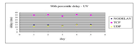
The performance of UV is just like that of CAM. All three protocols are very stable. The performance of UDP and TCP NODELAY are very close. The difference is less than 15%. The delay of TCP is about two to three times that of the other two protocols.
