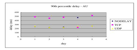
We can see that the delay of UDP and TCP NODELAY are very close. Both of them are much lower than that of TCP. The delay is around half of TCP's, and the jitter is only 15% of TCP's. However, on the fourth day, there is an exception. The delay of TCP NODELAY is much higher than that of TCP. However, the jitter is normal. This may be due to the heavy congestion of the network when we did the TCP NODELAY test. This shows that the network between Sydney and Columbia is not stable.
