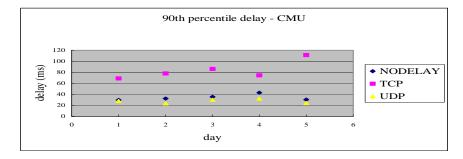
The delay for of CMU is worse than that for CAM, but better than that for Sydney. There is no exception for these three protocols. UDP and TCP NODELAY are very close. The difference is about 10% to 20% for delay. TCP has a much worse performance. Both delay and jitter are more than twice those of the other two protocols.
