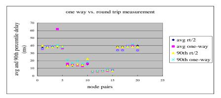
From both the chart and the data table, we can see that the results from these two measurements are almost the same. This proves that using the round trip measurement is as accurate as one-way measurement.
