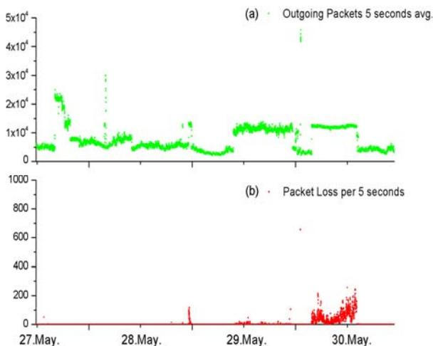
Figure 4. Outgoing Packets & Loss Distribution
