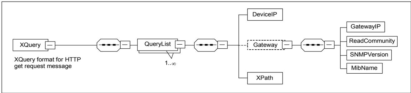
Fig. 6. XML Schema for “XQuery” in HTTP Get.
