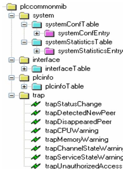
Figure 3. Structure of Common PLC MIB
