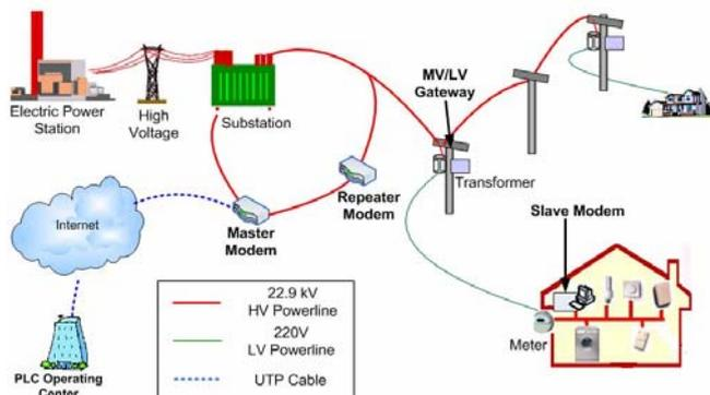
Figure 1. Structure of PLC Network
