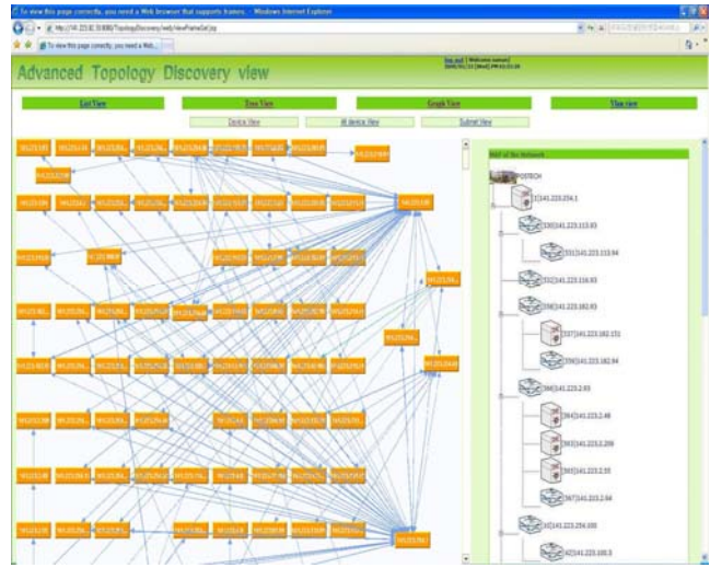
Fig. 2. Graph View of L3 and Tree View of L2 Devices in POSTECH
