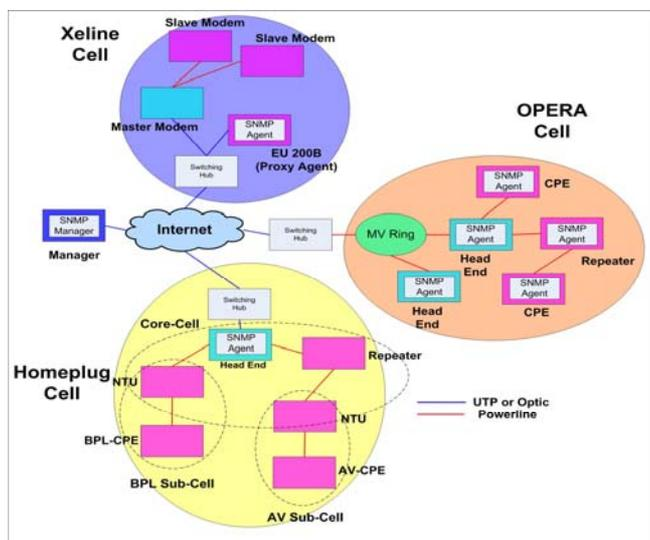
Fig. 1. Overall Architecture of Multi-vendor PLC network
