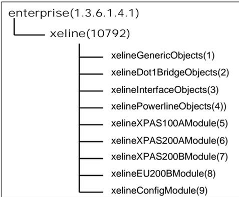
Fig. 2. Structure of Xeline PLC MIB
