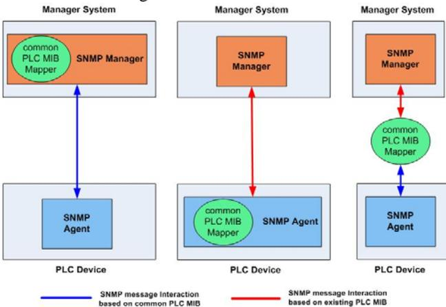
Fig. 7 Possible locations of common PLC MIB Mapper
