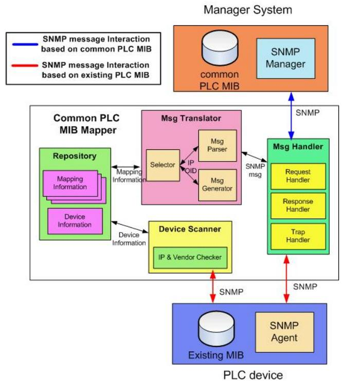
Fig. 8. Architecture of common PLC MIB Mapper
