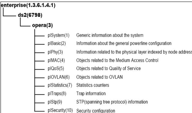
Fig. 3. Structure of OPERA PLC MIB
