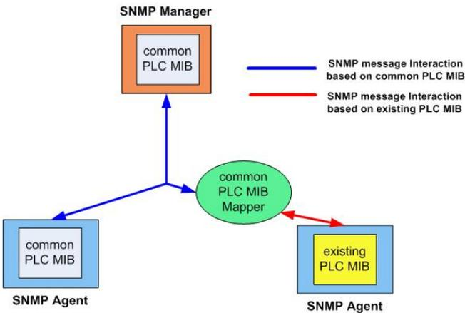
Fig. 6. Operation of common PLC MIB Mapper
