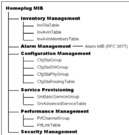
Fig. 4. Structure of Homeplug PLC MIB
