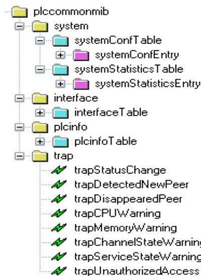
Fig. 5. Structure of Common PLC MIB
