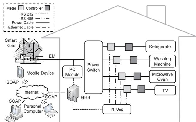
Fig. 1. Green Home Service Deployment in POSTECH for Smart Grid
